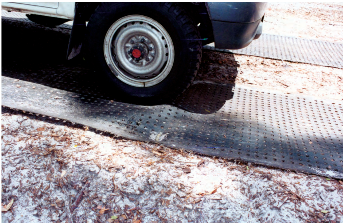
Photo #4. Holeybelt laid over a sandy track on Morton Island minimises the formation of wheel ruts. In this application the belt needs to be stretched somewhat and pegged down at the ends.
